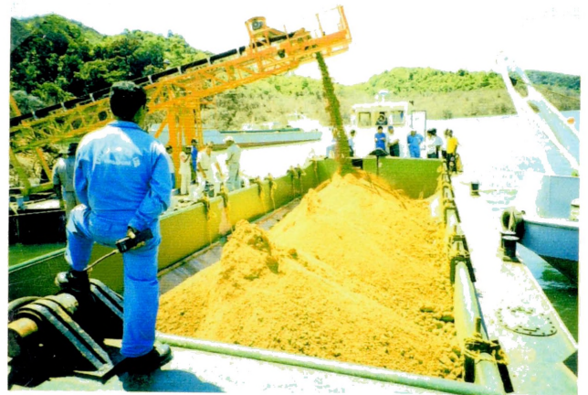
Loading Operation into Barge through Belt Conveyor provided on Pontoon
