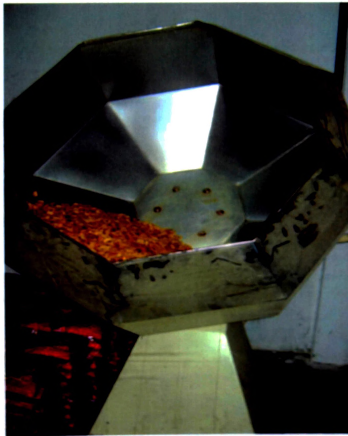
Figure 6:12 Flavoring drum – add vegetable oil, salt, chilly powder, garlic powder, Onion powder with biscuits
