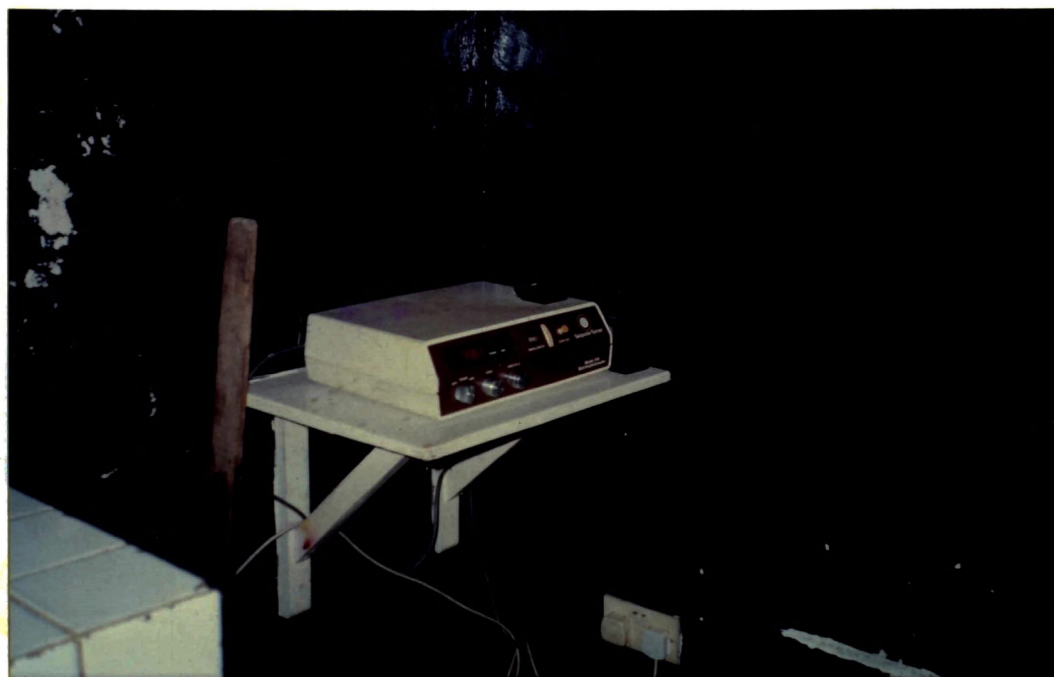
Figure 3.5 Colorimeter to determine the colour of sugar
