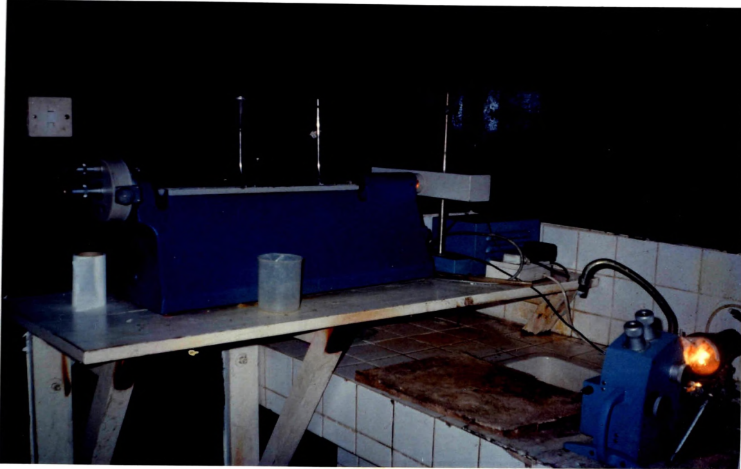
Figure 2.5 Polarimeter to determine pol value
