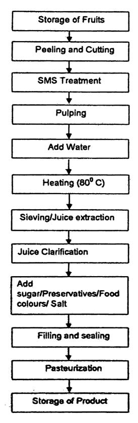
Figure 3.1: Manufacturing process
