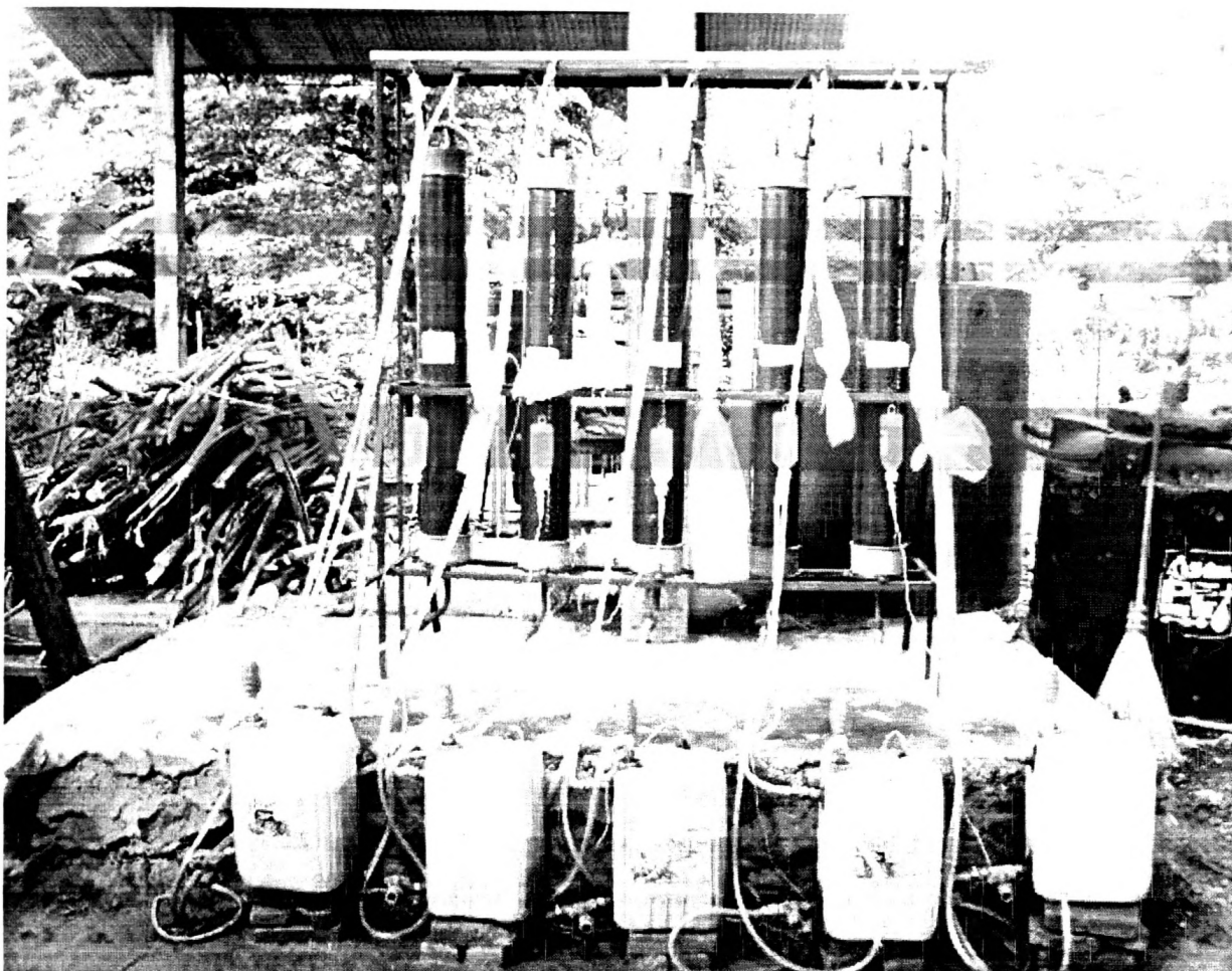
Figure 4.5 Designed leaching column structure for five types of wastes
