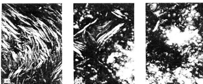
Figure 2.7 photomicrographs of Distilled Monoglycerides in (a) gel form, (b) partially recrystallized, (c) completely recrystallized to a coagel (Friberg, 1976).
