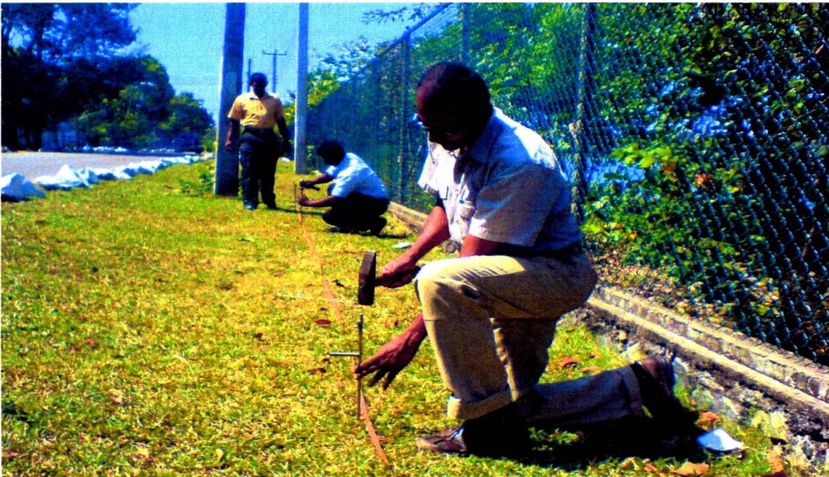
Figure 3.3: Placing electrodes on the ground prior to data acquisition. According to the theory, the electrodes were stationed on a straight line and water is added to maintain a proper contact with the ground.
