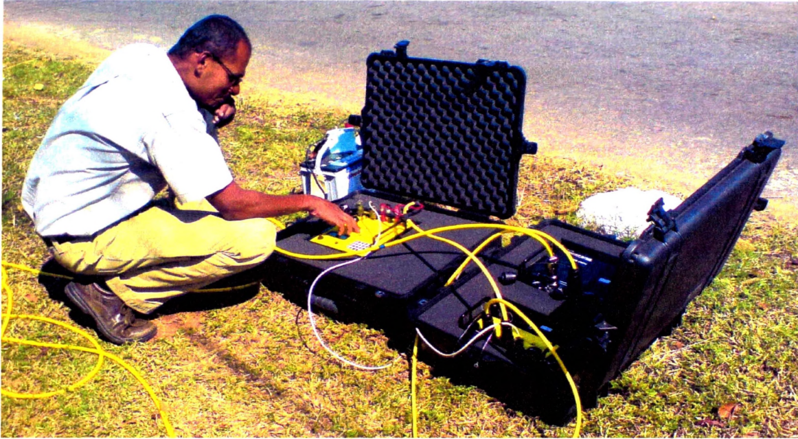
Figure 3.2: AGI resistivity imaging system that was deployed in the field for data acquisition and comparison purposes. Twenty-eight electrodes have been deployed along the same line where the 1D VES stations were places with an interval of 2m electrode spacing.
