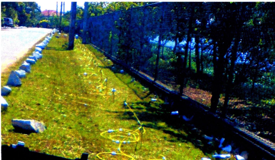
Figure 1.1: Selected stretch of land for fieldwork. Both 1D and 2D systems were deployed in the same stretch for data collection. 1D survey was conducted with 4m station spacing (details are given below) and the same stretch has been imaged with AGI 2d system at electrode spacing 2m with total of 28 electrodes.
