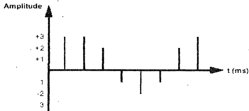
Figure 4.2: Samples with the corresponding quantised values
