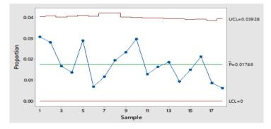
Reliable control limits, which were developed after removing the out-ofcontrol data points were shown in Figure 3 and the control limits are varying and are based on the number of registered students (number of each sample size). Central Line (CL) is .017746 (1.77%) which means that on average, 1.77% of students failed.
