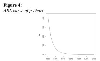
According to Figure 4 and Table 1, when the process is in control (hSigma = 0), the expected number of samples (436) before getting the first out-of-control signal is very high. As a result, ARL values are significantly large for small shifts in the process mean. In contrast, ARL values get smaller when there are considerably large shifts. Therefore, it shows that the performance of the developed p-chart is highly reliable in detecting out-of-control situations.
